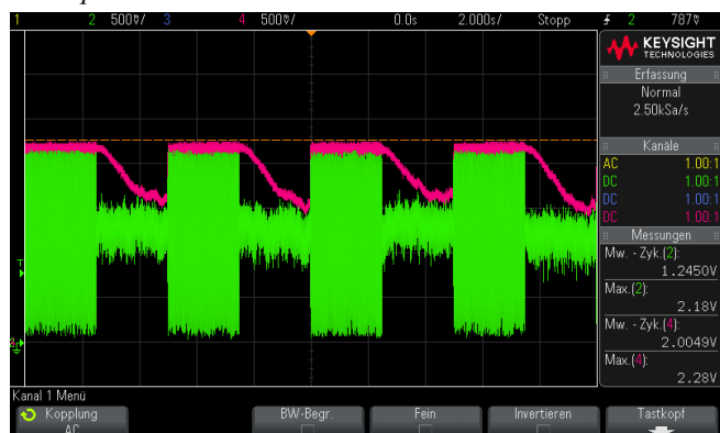
Fig. 6. Oscilloscope screen snapshot of the experimental results with the PGA output signal (green) and the envelope detector output signal (magenta).
